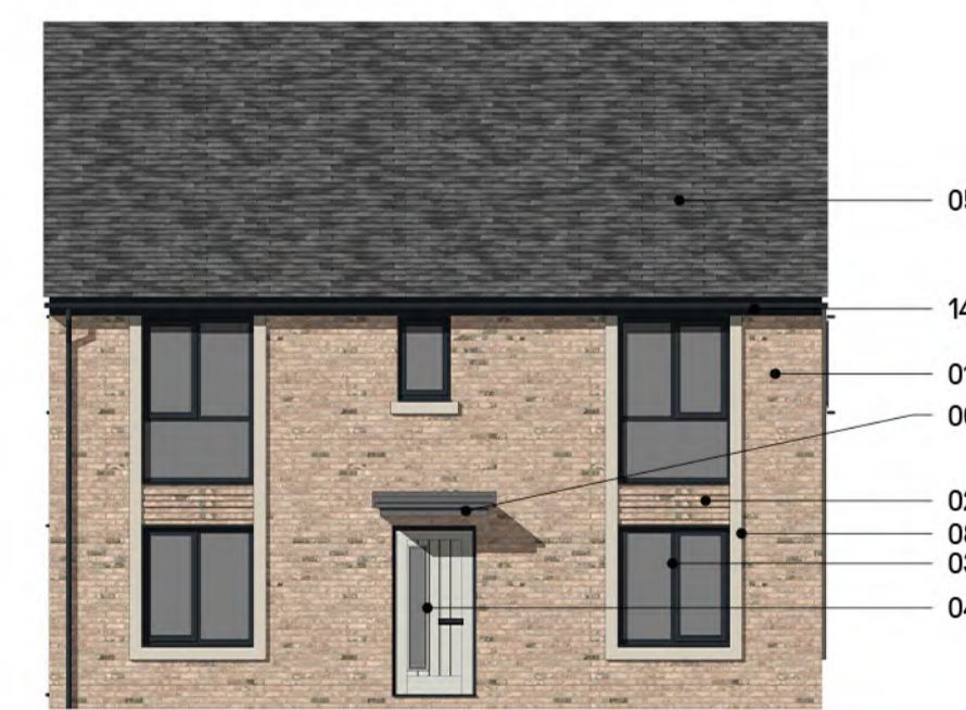
8 FRONT ELEVATION - A 1:100 APPLICABLE FOR PLOT 41 ONLY
